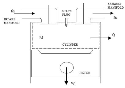
Figure 3. Engine Cylinder Thermodynamic System.
