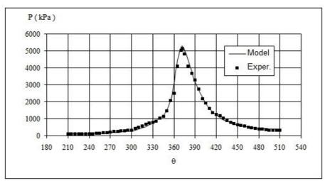
Figure 5. Comparison of Cylinder Pressure Predictions of Presented Model and Experimental Results from Taylor [10].
