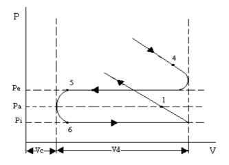
Figure 4. Gas Exchange Processes in the Engine Cylinder.
