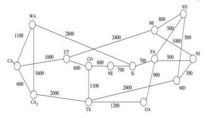
Figure 3. The 14-node NSFNET network topology showing approximate distances between the nodes in km.
