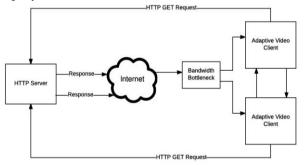
Fig. 2. Collaborative DASH-based Adaptive Video Streaming
