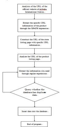
Figure 1Crawler crawling flowchart
