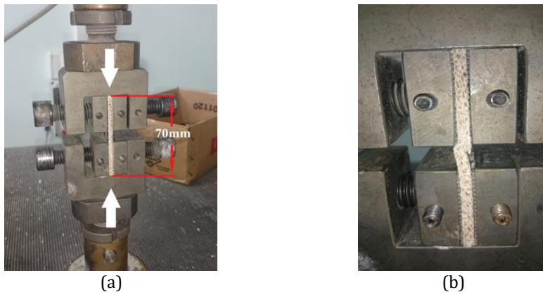
Fig. 5. (a) Compression test configuration and (b) compression damage
