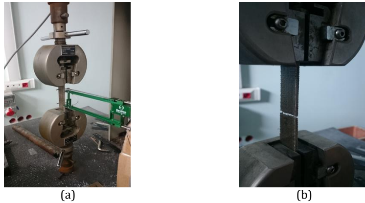
Fig. 4. (a) Tensile test configuration and (b) tension damage
