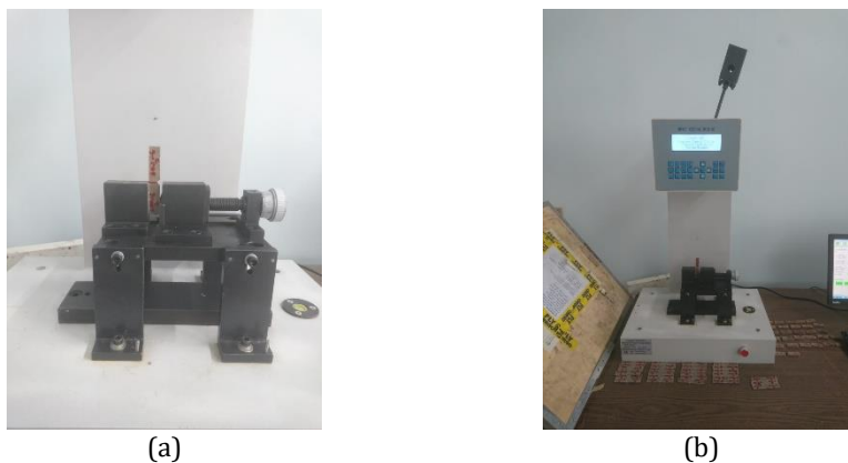
Fig. 6. (a) Impact test sample and (b) Izod impact test machine
