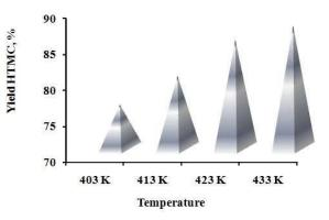
Fig. 2. The effect of temperature on the HTMC yield at the molar ratio of DMB:HEMA of 1.5:1
