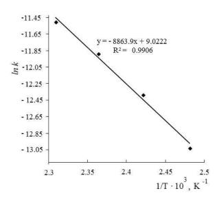
Fig. 5. Arrhenius dependence for the cycloaddition reaction between DMB and HEMA
