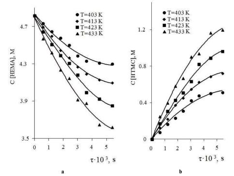
Fig. 3. Kinetic curves of HEMA consumption (a) and HTMC accumulation (b) at the molar ratio DMB:HEMA= 1.5:1 in the temperature range of 430–433 K
