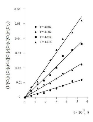
Fig. 4. Linearized kinetic curves for the HEMA consumption in the temperature range of 403–433 K at the molar ratio DMB:HEMA=1.5:1
