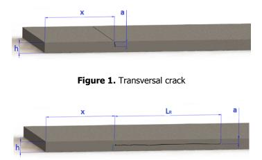
Figure 2. Longitudinal crack
