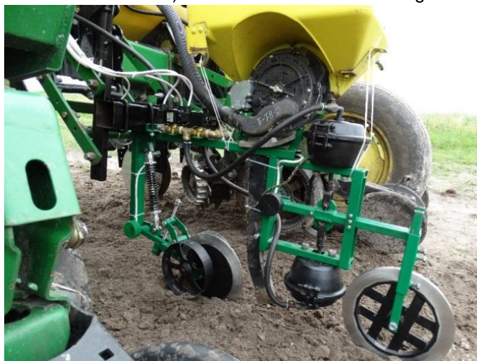
Fig. 6 - A two-phase coultter system on John Deere 7000 planter
