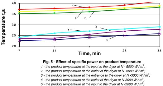
6 - the product temperature at the outlet of the dryer at N -2000 W /  $m^2$ ;
