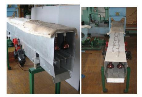
Fig. 2 - Photo of experimental vibrotray infrared dryer (*impeller*, outlet pipes, regulating sider on the photo not shown)
