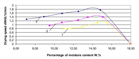
Fig. 4 - Effect of specific power on the drying speed  $1 - N = 2000 W/m^2$ ;  $2 - N = 3000 W/m^2$ ;  $3 - N = 5000 W/m^2$ .
