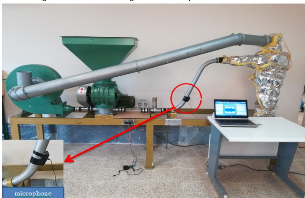
Fig 1 - Schematic of wheat grains conveying system and acoustic signals recording system
