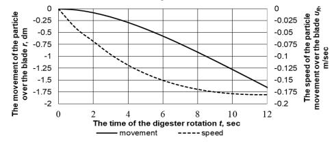
Fig. 5 - The dependence of the movement over the digester blade and the speed of the organic particle on the rotation time (angular velocity of the digester rotation  $\omega$ =0.1 rad/s, inner radius *R*=2 dm)
