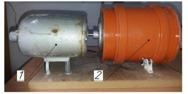
**Fig. 3 - Research plant** 1 – electric drive, 2 –the body of the plant (horizontal cylinder)
