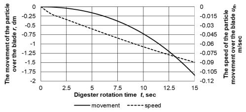
Fig. 4 - The dependence of the movement over the digester blade and the speed of the mineral particle on the rotation time (angular velocity of the digester rotation ω=0.1 rad/s, inner radius *R*=2 dm)
