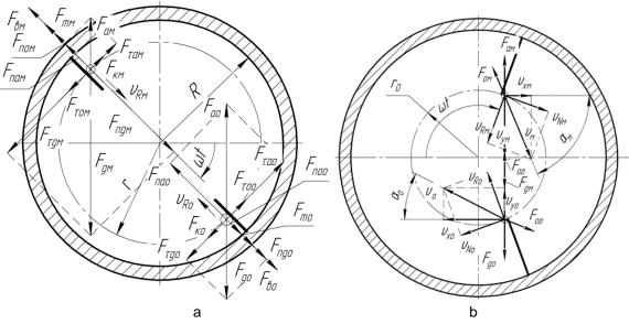
Fig. 2 - Scheme of action of forces on mineral (*M*) and organic (*O*) substrate particles (a – when interacting with the blades, b – in free movement)
