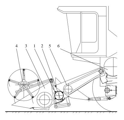
**Fig. 1 - General view scheme of a combine harvester header with a device for preliminary grain threshing:** 1 – a tooth and spatulate shaped thrashing drum; 2 – a deck; 3 – a header; 4 – a reel; 5 – an inclined chamber conveyor; 6 – threshing-separation system of combine harvester
