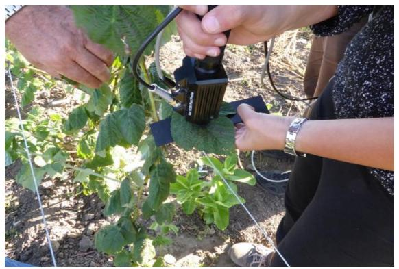
Fig. 6 - Contact reflectance measurement with PlantProbe
