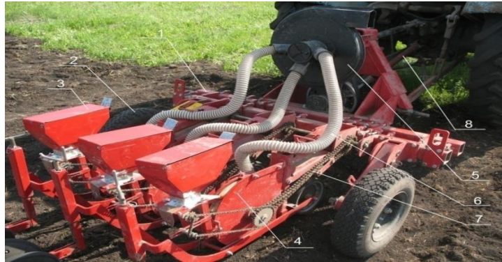
Fig. 8 – General view of the planting machine equipped with vibration-pneumatic planting device 1 – frame; 2 – support wheel; 3 – bunker; 4 – planting section; 5 – the fan; 6 – vacuum line; 7 – a chain; 8 – prop shaft
