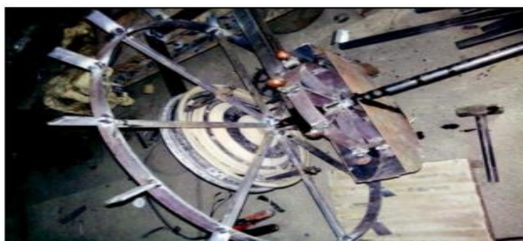
Fig. 3 – Disk seeder with diametrically located blades
