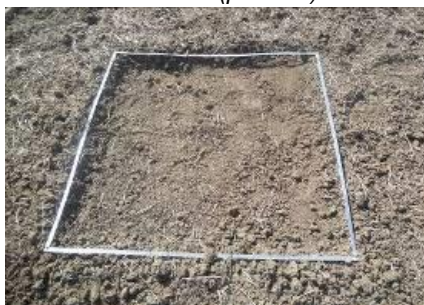
Existing soil mass on the soil surface (per 1m 2 ) after the cultivator-tractor aggregate has passed
