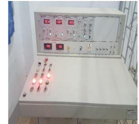
Figure 3: HV 9103 control desk includes measuring instruments and trigger device.
