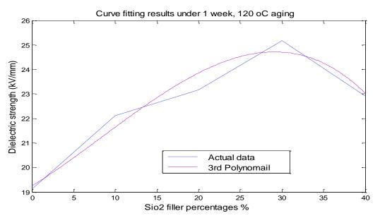
Figure 9: Effect of filler addition on dielectric strength after one-week aging at 120 °C.
