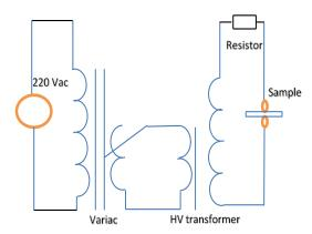
Figure 4: Schematic diagram for dielectric strength testing circuit.
