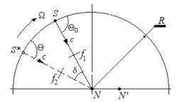
Figure 14: Inertial reference system.  $f_1$  is wave front from the source in its reference frame;  $f_2$  is distorted wave front, perceived by the observer.
