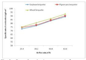
Fig. 3 : Rate of combustion w.r. to air flow rate of crop residues briquette.
