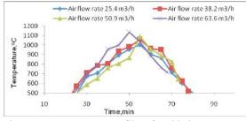
Fig. 8 : Temperature profile of oxidation zone with mix biomass briquette.
