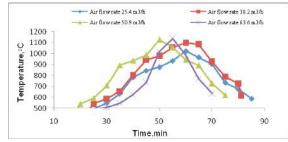
Fig. 7 : Temperature profile of oxidation zone with pigeon pea briquette.
