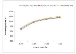
Fig. 4 : Oxidation temperature of briquette at different air flow rate.
