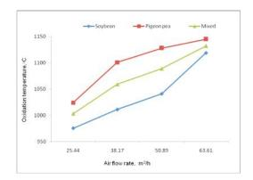
Fig. 5 : Flame temperature with briquette at different air flow rate.
