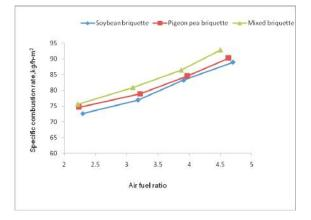
Fig. 2 : Specific rate of combustion of briquette of different biomass.
