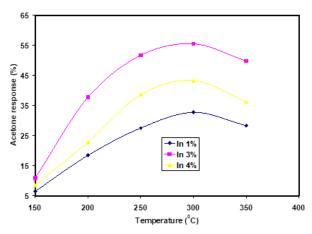
Fig. 1: Acetone response of In: ZnO film 1000 ppm acetone at different temperatures.
