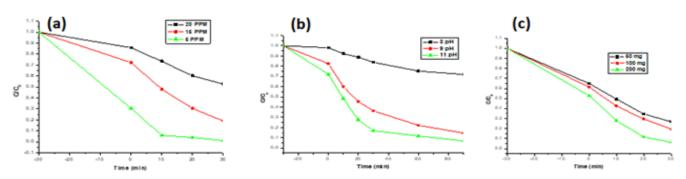
**Fig. 3.** (a) Effect of concentration of MB; (b) Effect of different pH on depredation of MB; (c) Effect of different wt. of catalyst on degradation of MB
