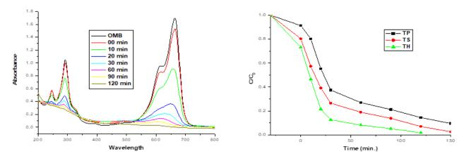
**Fig. 2.** Photocatalytic degradation of MB by  $TiO_2$  sample (HT method) and Kinetic parameter study of degradation of MB by different  $TiO_2$  samples.
