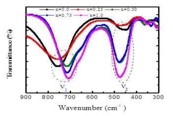
Fig 2: Infrared spectra for the series Pr<sub>x</sub>CoFe<sub>2-x</sub>O<sub>4</sub>.
