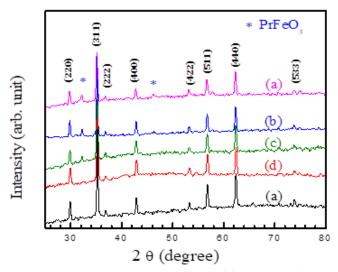
Fig. 1: X-Ray diffraction patterns of (a) x = 0.0, (b) x = 0.025, (c) x = 0.050, (d) x = 0.075 and (e) x = 0.1 for  $Pr_xCoFe_{2-x}O_4$
