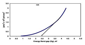
Fig. (C) Energy band gap of semiconductor CdS thin film
