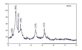
Fig (a) XRD Pattern of CdS thin film
