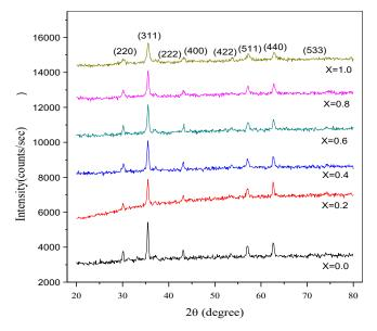
**Fig.1.** X-ray diffraction patterns of the  $CuCr_xFe_{2-x}O_4$  (x = 0.0, 0.2, 0.4, 0.6, 0.8, 1.0) nanoparticles
