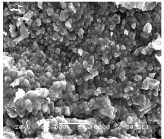
Fig. 3: Typical SEM image (x=0.6) of  $CuCr_xFe_{2-x}O_4$  nanoferrite system
