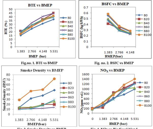
Fig. 3. Smoke Density vs BMEP
