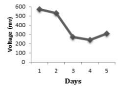
For domestic waste, zinc was used as anode and cathode. The parameters and electricity generated were measured.
