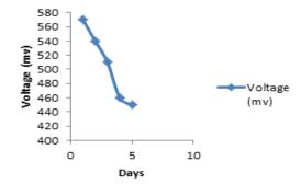
2] **Dairy Waste:** For dairy waste, zinc was used as anode and copper as cathode. The parameters and electricity generated were measured.
