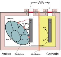
Fig.1: Microbial fuel cells
