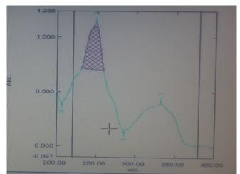
**Fig 6:** .Area between 229-260nm selected for pazufloxacin mesylate (10µg/ml)
