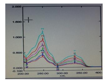
Fig.3: Overlay of spectra of Pazufloxacin Mesylate
