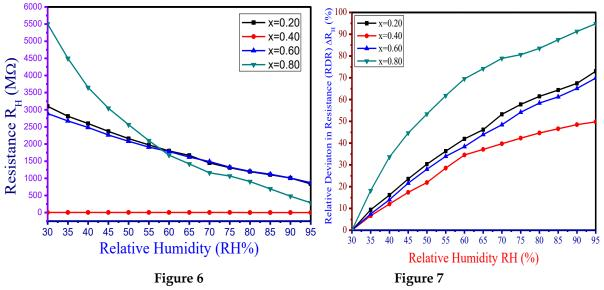
**Figure 6:** Graph of Resistance ( $R_H$ ) against applied relative humidity (%RH) for thick film of compositions of Ni<sub>x</sub>Zn<sub>1-x</sub>Fe<sub>2</sub>O<sub>4</sub> nanoferrites deposited on ceramic substrate
