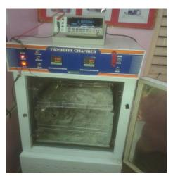
**Figure 1:** Experimental arrangement for measurement of humidity dependent characteristics of the composition under investigation.
