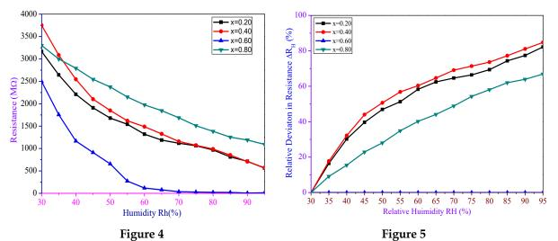
**Figure 4:** Graph of Resistance ( $R_H$ ) against applied relative humidity (%RH) for thick film of compositions of  $Mn_xZn_{1-x}Fe_2O_4nanoferrites$  deposited on ceramic substrate
