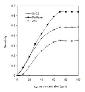
**Fig.(4)**:Variation of sensitivity with of  $CO_2$  gas concentration at room temperature.
