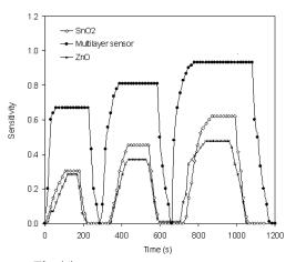
Fig.(6): Static response of pure SnO<sub>2</sub>, pure ZnO and Multilayer sensor at room temperature
