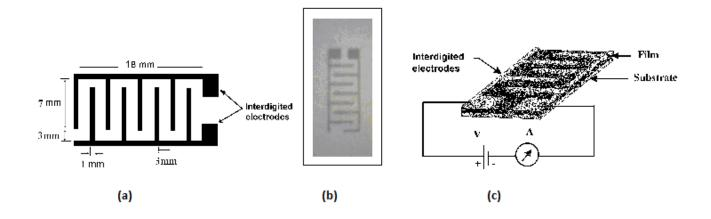
**Fig. 1**:(a) Fabrication of interdigited Electrodes (b) Actual photograph of interdigited electrodes (c) Circuit of resistance measurement using interdigited electrodes.
