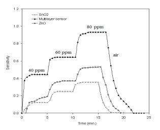
**Fig.(5)**:Dynamic response of pure SnO<sub>2</sub>, pure ZnO and Multilayer sensor at room temperature.
