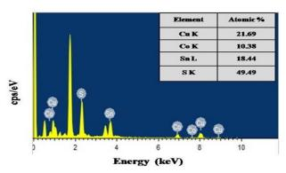
Fig.4- EDAX spectrum of CCTS film deposited at 350 °C
