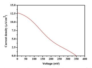
**Fig.6-** Current density-voltage (J-V) characteristics of the CCTS based photoelctrochemical solar cell
