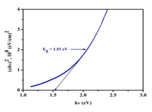
**Fig.5**- Plot of  $(\alpha hv)^2$  versus hv of CCTS film deposited at substrate temperature 350 °C
