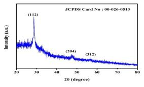
Fig.2 -XRD pattern of CCTS thin film deposited at a substrate temperature of 350  $^{\circ}\mathrm{C}$
