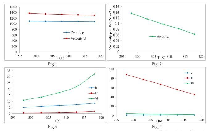
**Fig 1**: Variation of Ultrasonic velocity U (m/sec) and density  $\rho(Kg/m^3)$  with temperature T (K) **Fig 2**: variation of viscosity  $\eta$  with temperature T(K) **Fig 3**: Variation of adiabatic compressibility  $\beta$ , free length L<sub>f</sub> and free volume V<sub>f</sub> of mixture with temperature **Fig 4**: Variation of acoustic impedance Z, relaxation time  $\tau$  and internal pressure  $\pi$  of mixture with temperature
