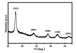
**Figure 1**. The X-ray diffraction (XRD) pattern of pure  $TiO_2$  NPs film
