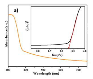
**Figure 3**. UV-visible spectrum of TiO<sub>2</sub> NPs film (inset: Tauc plot- variation of  $(\alpha h \upsilon)^2$  versus photon energy,  $h \upsilon$  (eV))
