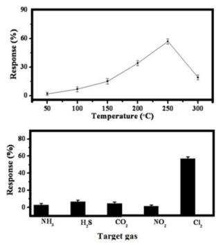
**Figure 4**. The variation of sensor response at different operating temperatures for  $TiO_2$  NPs film at 100 ppm of  $Cl_2$  target gas (Top) and sensor response for  $TiO_2$  NPs film at 100 ppm for different test gases.
