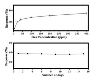
**Figure 5**. Variation of  $TiO_2$  NPs film sensor response at different concentration (ppm) of  $Cl_2$  target gas (top) and variation of  $TiO_2$  NPs film sensor response at 100 ppm of  $Cl_2$  target gas at different time intervals (bottom)
