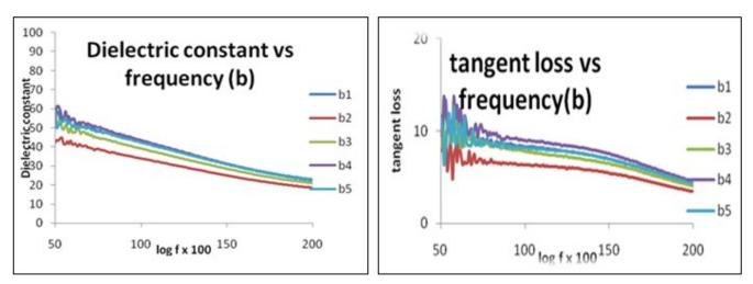
Figure 3A: Variation of dielectric constant with frequency. Figure 3B: Variation of tangent loss with frequency.
