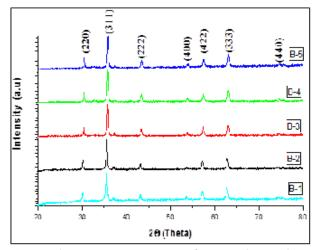
**Fig.1.** Shows XRD pattern for synthesized Nio.<sup>5</sup>  $Co_{0.5}Nd_xFe_{2-x}O_4$  samples with varying Nd concentration from B-1) 0.025, B-2) 0.05, B-3) 0.075, B-4) 0.1, and B-5) 0.125.
