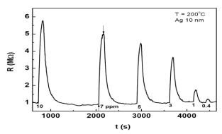
**Figure 4** shows the response curve recorded for the sensor film when it is subjected to decreasing concentrations of NO<sub>2</sub>.
