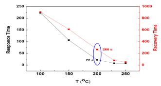
**Figure 3.** Response and recovery times as a function of operating temperature recorded for sensor film with 10 nm of Ag upon exposure to 5 ppm of NO<sub>2</sub> at 200°C.
