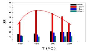
**Figure 2.** Sensor response as a function of operating temperature and Ag thicknesses.
