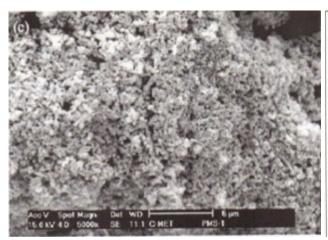
**Fig. 4** SEM Image of 28 min. electochemically oxidized Tl-Ba-Ca-Cu alloyed Films
