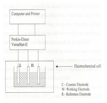
Fig.1 Electro-deposition set up
