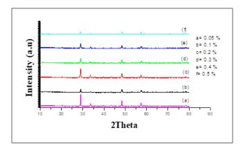
**Fig.1:** XRD patterns of  $(Y_{1-x} \text{ Gd }_x)_2O_3$  prepared by HCP method with variable concentration of dopant (x= 0.05 to 0.5 %)
