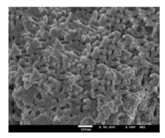
**Fig.2:** SEM image of  $Y_2O_3$ : Gd <sup>3+</sup> (x= 0.2 %) phosphor prepared by HCP method.
