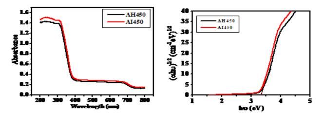
Fig 3. UV-Visible spectra and corresponding Tauc plots for AH450 and AI450 TiO<sub>2</sub> powders
