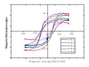
**Figure 2**. Hysterisis loop of Co1-xPbxFe2O4 where x = 0.1, 0.2, 0.3, 0.4, and 0.5after sintering at 600°C
