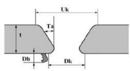
Fig.3. Kerf geometry of an AWJ cut
