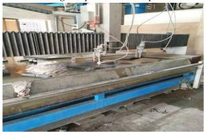
Fig2: Water jet Machine
