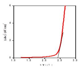
Fig 4. Optical absorption spectra of CdS thin film
