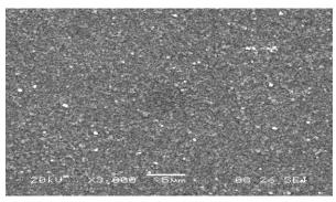
Fig : SEM image of CdS thin film
