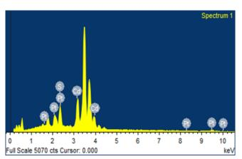
Fig 3. EDS of CdS thin film
