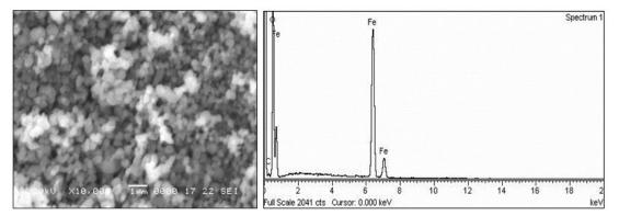
Fig. 3: SEM Image of Iron oxide Nanoparticle
