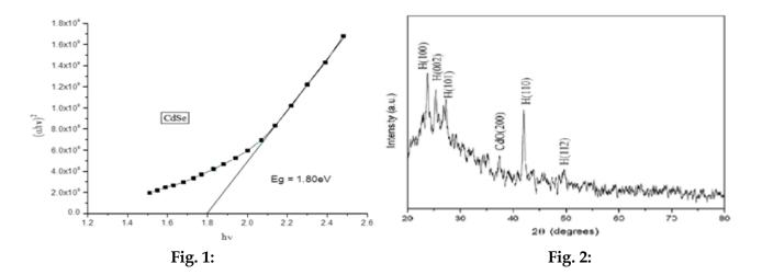
Fig. 1: Variation of  $(\alpha hv)^2$  vs. Photon energy (hv) at temperature 300 °C Fig: 2. XRD patterns of CdSe thin films deposited at substrate temperatures of 300°C
