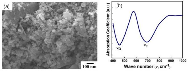
Figure 2 (a) FE-SEM image and (b) FT-IR Spectrum of Cobalt Ferrite nanoparticles
