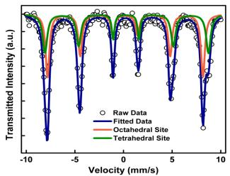
**Figure 4** Mössbauer spectrum of cobalt ferrite nanoparticles.
