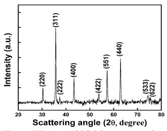
Figure 1. XRD pattern of Cobalt ferrite nanoparticles
