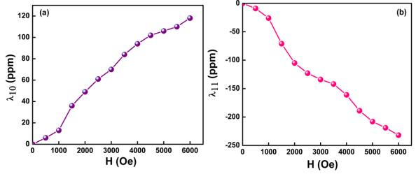
**Figure 3.** Magnetostriction as a function of magnetic field recorded in the **(a)** perpendicular direction ( $\lambda_{10}$ ) and **(b)** parallel direction ( $\lambda_{11}$ ) to the applied magnetic field.
