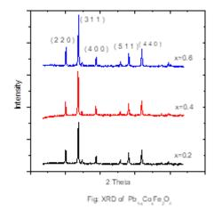
Figure 1: shows the XRD pattern of Pb<sub>1-x</sub>Co<sub>x</sub>Fe<sub>2</sub>O<sub>4</sub>
