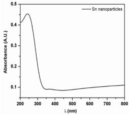
**Fig 3:** The UV visible spectrogram of synthesized Sn nanoparticles
