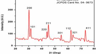
Fig 2. XRD spectra of synthesized Sn nanoparticles.
