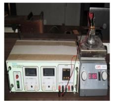
Fig 1. Electro-deposition Setup in the laboratory
