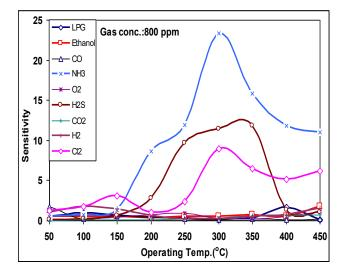
**Figure.3** Variation of sensitivity with operating temperature.
