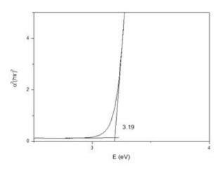
Figure 2: UV-DRS absorption Tauc plot of Zn<sub>2</sub>TiO<sub>4</sub>
