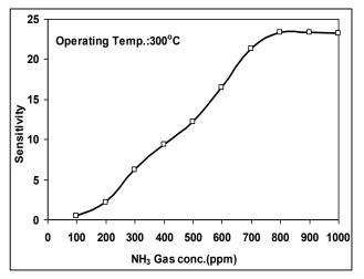
**Fig. 4:** Dependence of the sensitivity of the  $Zn_2TiO_4$  thick film on the NH<sub>3</sub> concentration at 300 °C
