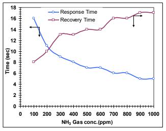
**Figure 6.** Variation of response and recovery time with concentration of NH<sub>3</sub>.
