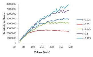
Fig.4: Graph of dc Resistivity with Voltage at 200°C
