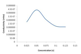
Fig.5: Graph of dc conductivity with concentration (x) at  $200^{\circ}$ C
