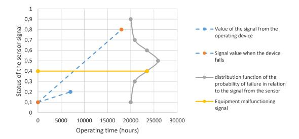
**Fig. 6.** Graphical method for determining the input data for calculating the average operating time of the equipment, depending on the diagnostic signals from the sensors *Source:* compiled by the authors.
