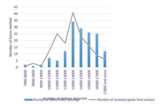
**Fig. 5.** The number of defects that occur depending on the running time of the electric motor *Source:* compiled by the authors.
