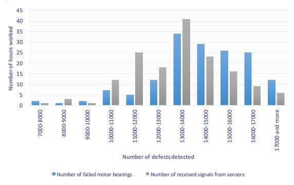
**Fig 4.** The number of defects that occur depending on the running time of the electric motor *Source:* compiled by the authors.
