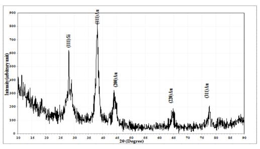
Figure 3- X-ray diffraction pattern of Au NPs at laser energy 800 mJ/pulse.
