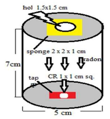
Figure 1- Radon monitors "Can technique".
