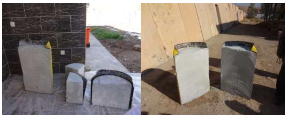
Figure 1- Low magnification optical graphs of cut open conditioned solid wasteContainer.
